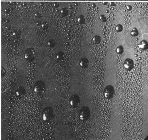
FIG. 1. The appearance of dropwise condensation at different heat fluxes.
